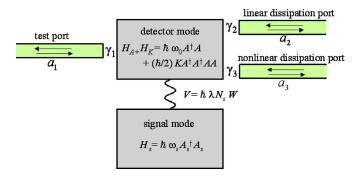
FIG. 1. (Color online) The model includes nonlinear detector mode coupled to three ports, a test port, a linear dissipation port, and a nonlinear one, and a linear signal mode coupled to the detector mode.
