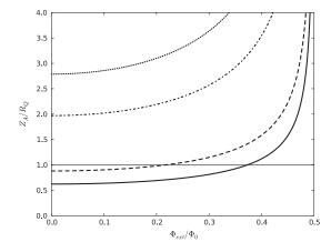
FIG. 3. Ratio of array impedance  $Z_A$  to the resistance quantum  $R_Q$  as a function of the external flux bias for a critical current  $I_c=2~\mu{\rm A}$  and example ground capacitor values:  $C_0=10^{-16}$  (solid line),  $5\times 10^{-17}$  (dashed line),  $10^{-17}$  (dash-dotted line), and  $5\times 10^{-18}$  F (dotted line). High- and low-impedance regions are defined above and below  $Z_A/R_Q=1$ , respectively.
