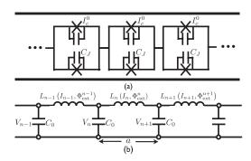
FIG. 1. (a) Layout of the dc-SQUID transmission line. We assume each SQUID element is formed from identical tunnel junctions with critical current  $I_c$  and capacitance  $C_J$ . (b) Effective lumped circuit model valid for frequencies below the plasma frequency and negligible SQUID self-inductance.
