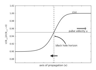
FIG. 2. Effect of a steplike flux pulse on the propagation velocity of a JJA as seen in the comoving frame. The pulse velocity was chosen to be u=0.95c ( $\Phi_{\rm ext}=0$ ). The black hole horizon occurs where c(x)=u. The arrow indicates the only permissible direction of travel across the horizon.
