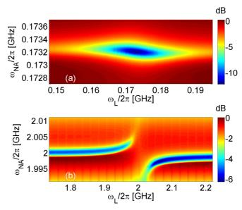
FIG. 3. ESR of (a) the omega and (b) the spiral resonators. The color-coded plots display the measured reflectivity coefficient  $|S_{11}|^2$  vs  $\omega_{\rm L}$  (i.e., vs static magnetic field) and the probing frequency  $\omega_{\rm NA}$ . Measurements are performed by a network analyzer at a temperature of T = 3.1 K, for which the polarization coefficient  $p_0$  [see Eq. (A20)] is given by  $p_0 = -1.4 \times 10^{-3}$  ( $p_0 = -1.6 \times 10^{-2}$ ) for the omega (spiral) resonator.
