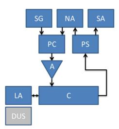
FIG. 2. The experimental setup. A power combiner (PC) is employed for combining the injected signals of a signal generator (SG) and a network analyzer (NA). The combined injected signal is transmitted through an amplifier (A) and a coupler (C), and feeds the loop antenna (LA), which is positioned above the device under study (DUS). The back-reflected signal is split by a power splitter (PS) and measured by both a NA and a spectrum analyzer (SA).
